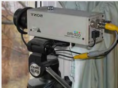
Sony CCD-IRIS Colour camera on tripod Auto-Iris 25mm F1.3 Lens
